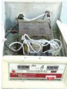
Fig: 16.20 Transformer in stabilizer
