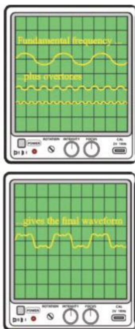
Fig: 11.6 Formation of a note on the oscilloscope
