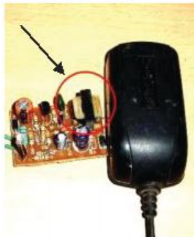
Fig: 16.21 Transformer battery charger
